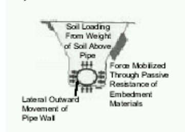
Figure 1. Mobilization of Enveloping Soil Through Pipe Deformation
